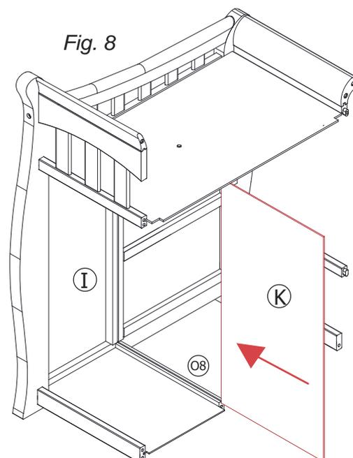
4. Put the Right Ends on ground, then Insert Middle Panel (K) into Right End (I), See Fig. 8
