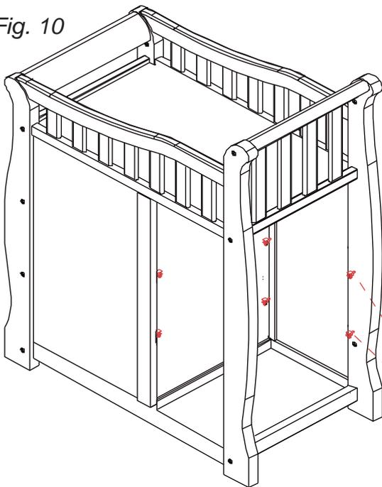
7. Insert Shelf Support Brackets (HH) into holes in back of dresser, See Fig10.
