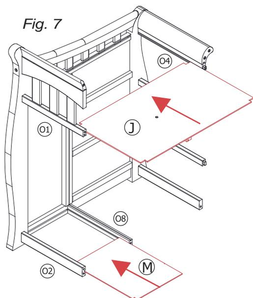
3. Slide (M) into grooves of O2 and O8
