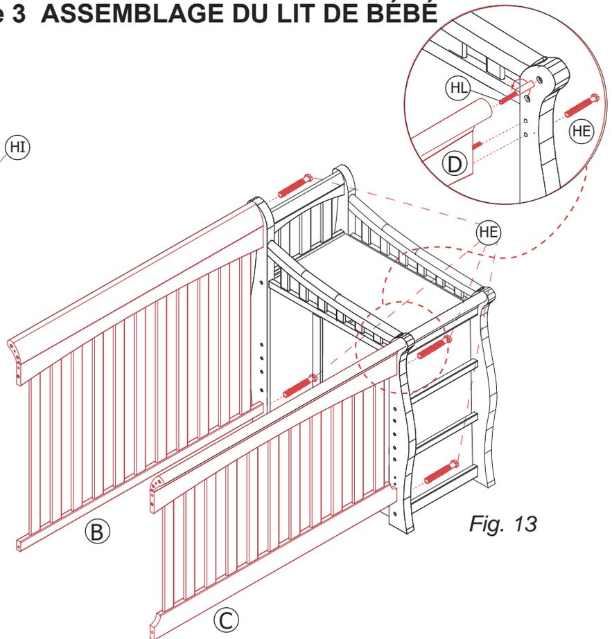
1. Slide 1 Wood Dowel(HI) into each end of Front & Back Frame (B&C). See Fig.12
