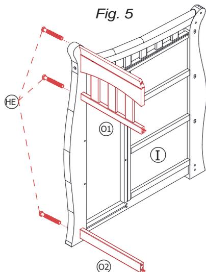
1. Slide 1 Wood Dowel(HI) into each end of Parts (O1&O2), Then attach Decorative Support Bar(O1) and Back Support Bar (O2) to Right End (I) using 3 Bolts(HE). See Fig.5
