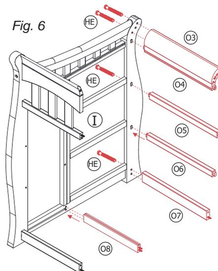
2. Slide 1 Wood Dowel(HI) into each end of Part (O7) and 2 Wood Dowel(HI) into each end of Part (O8). then Insert Contoured top(O3)&Support Bar O4;O5;O6;O7 and O8 into Right End (I) using 4 Bolts (HE) See Fig. 6
