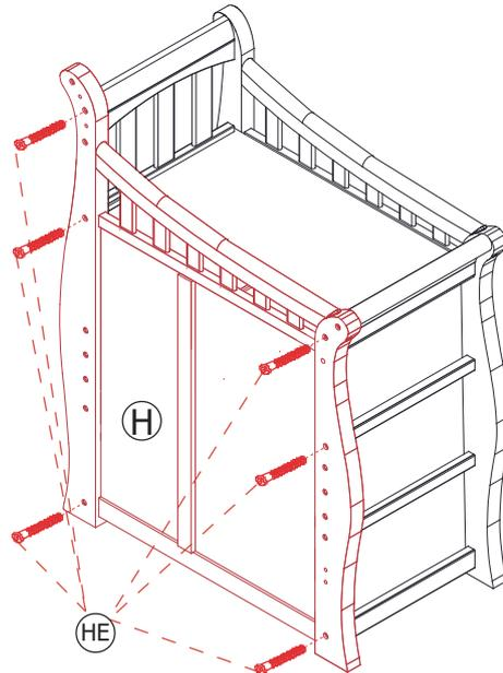
6. Attach Middle Panel(H) with each support bar and secure with 6 Bolts (HE). See Fig 9.
